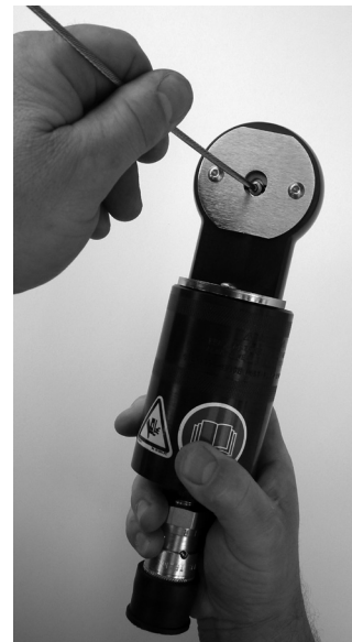
610 Portable Swager for use with 1/8" and 3/16" diameter cable.
