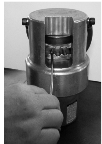
650 Portable Swager for use with all sizes of cable.
