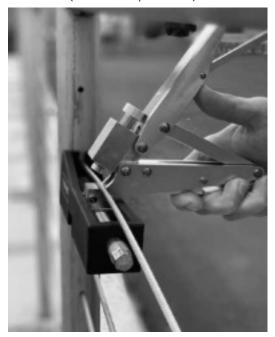
**2.** Adjust the brass-tip bolt to securely hold the cable. Lock the clamp.
