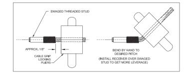
5. Install the Receiver in the post, following the instructions for installing Invisiware® Receivers at Post B in the "Installing Cable" on pages 4-9. When tensioned, the cables will self-align with the fitting at the other end of the cable run.
