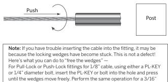
until the wedges move freely. Perform the same operation for a 3/16" Pull-Lock or Push-Lock, except use a 16d nail or another tool with 1/8" or smaller diameter. Anything larger than what is recommended can actually get stuck inside the fitting – NOT what you want!
