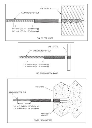
2. Slide the Body onto the cable and swage the Ferrule onto the end of the cable (see "Swaging Instructions," pages 15-16).
