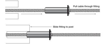
**5.** Hold the cable with one hand and slide the Pull-Lock fitting into the hole in the post. Press on the back of the Pull-Lock fitting to hold it securely in the post and pull the cable through the fitting until it is as tight as you can make it.
