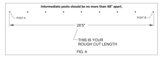
2. Measure out cable on a relatively clean surface (see Figure B below). A lawn or swept concrete surface would be fine. Cut cable to length using Cable Cutter.
