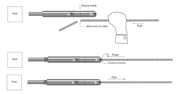
**4.** After successfully attaching the non-tensioning fitting, tension cable by holding tensioner body at 3/8" wrench flat nearest cable (do not let this section rotate while cable is inserted) and rotating female threaded section of fitting with a 3/8" open-end wrench onto threads.
