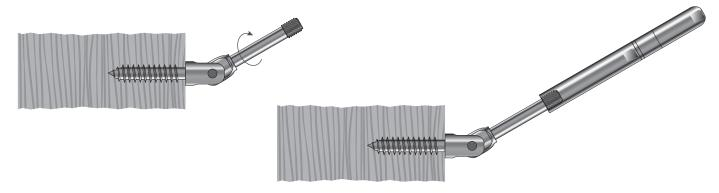
**2C.** If you are using the Push-Lock Tensioner with Threaded Bolt, hand turn the threaded bolt component of the assembly clockwise into the post, tightening with a 3/16" hex wrench. Assemble female threaded rotating portion of fitting onto male thread only so far as to cover the male thread and no more.
