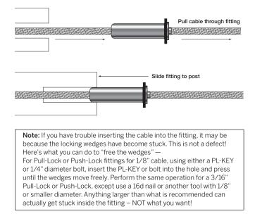
**6.** Hold the cable with one hand and slide the Pull-Lock fitting into the hole in the post. Press on the back of the Pull-Lock fitting to hold it securely in the post and pull the cable through the fitting until it is as tight as you can make it.
