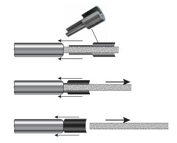
**4.** Remove the PL-Key and the jaws will reset to their original position, ready to accept and grip the cable again.
