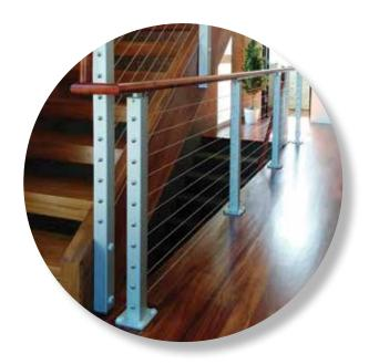
engineered to perform satisfactorily when subjected to the tension encountered when multiple load points (cables) are attached and tensioned properly to your end posts (225 lbs. per line). Center-to-center spacing of the cables vertically on the end posts should not exceed 3" spacing between the cables to allow for cable flex within the allowable limits to meet code requirements that a 4" sphere shall not pass through at any point.
